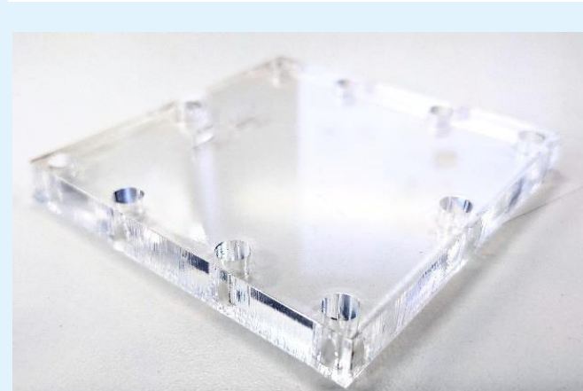
CAD model of part (top) and laser cut part (bottom). No additional finishing steps needed.
